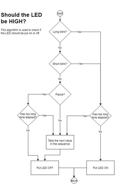
The function will ultimately result in putting the LED off after successful operation, regardless of it being short or long blink / pause, once too long time has elapsed. The next character value in the sequence is picked and LED is put off.
