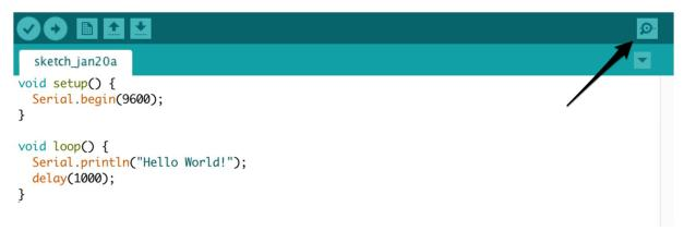
It opens a new window that displays messages from the Arduino, if the communication speed is set according to the settings in Arduino. Here it is 9600 bps. Whenever you suspect potential errors in your code, you can send simple texts through
