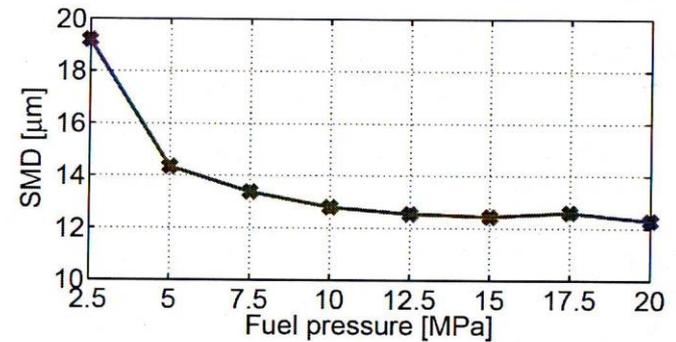
Figure 13. Influence of fuel pressure on the Sauter mean diameter (D32) of droplets in the spray core. Measurements taken in a heated spray chamber under evaporating conditions (1 MPa/600 K) [78].
