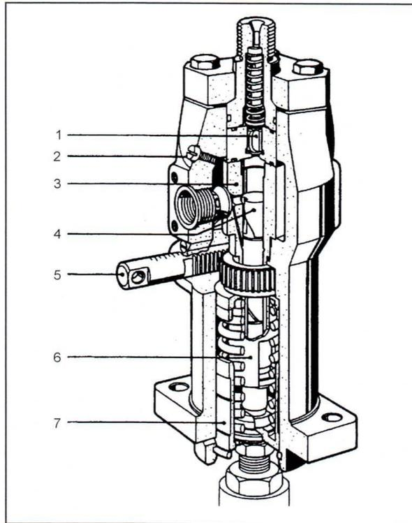
**Fig. 12-29** Mechanically controlled single-plunger fuel injection, individual injection pump for large engines<sup>6</sup>: 1, Pressure valve; 2, Vent screw; 3, Pump cylinder; 4, Pump piston; 5, Control rack; 6, Control sleeve; 7, Guide bushing.
