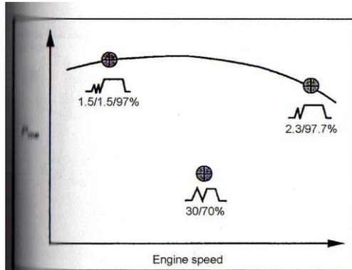
Fig. 12-25 Example of optimum, operation-point-dependent multiple injections in the engine map; quantity distribution in percent.<sup>5</sup>
