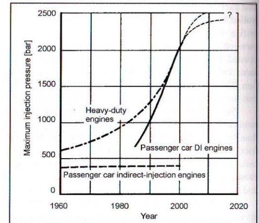
Fig. 12-21 Development of the maximum injection pressure in recent decades.
