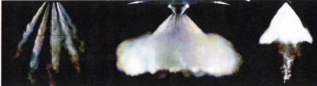
Figure 15. Examples of sprays from three types of injectors: left, multi-hole; center, outwards opening A-nozzle; right, an inwards opening swirl type nozzle. Note that the images are not taken using the same geometrical scale.
