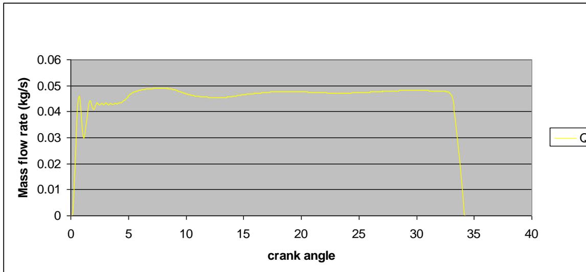
**Computed mass flow rate in the nozzle hole**
