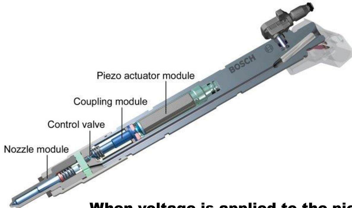
**When voltage is applied to the piezo stack (actuator module), its size increases ( $\sim 60\mu\text{m}$ ). Piezo injectors are very fast ( $<100$  micro-s), light, and consume low amount of energy.**
