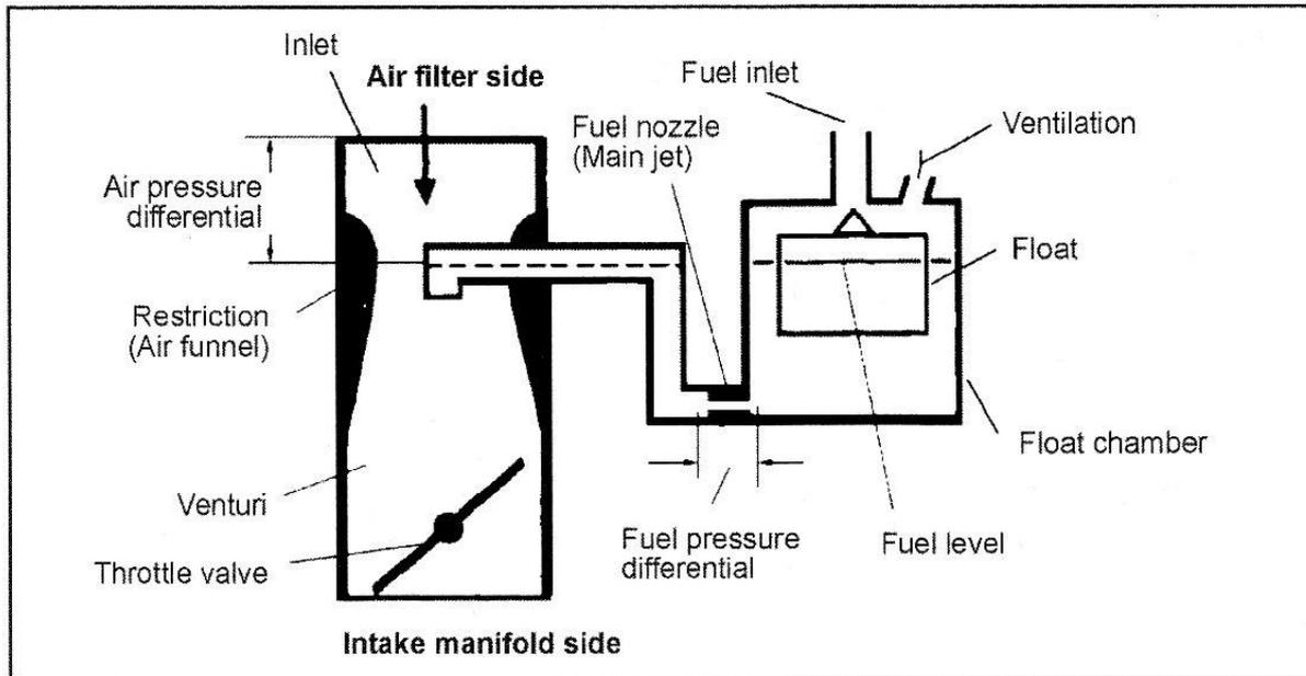
**Fig. 12-1** Functional principle of the carburetor.
