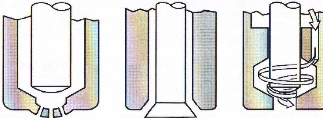
Figure 16. Cross-sections of three types of injector; left, multi-hole; center, A-nozzle; right, inwards opening swirl type nozzle. Reprinted with permission from SAE Paper No. 980498 [30], © 1998 SAE International.
