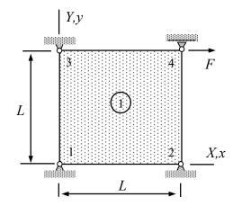
The spring force of non-linear spring depends on the dimensionless displacement a = u/L according to  $F = k(a - a^2 + a^3/3)$ . Determine the dimensionless displacement a = u/L if force F = k/4.
