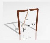
Pendulum with mass m = 1, pole length L = 1 and random force w(t):
