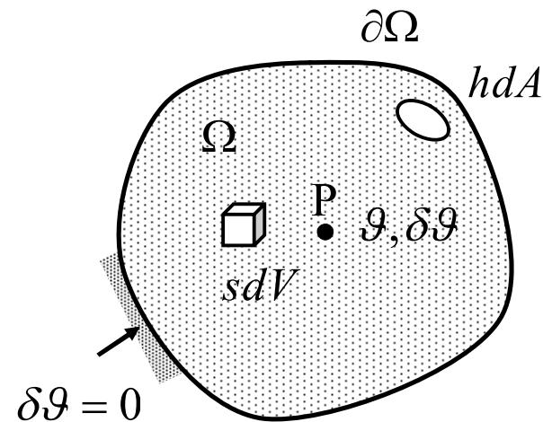
Finite element method is applied in the usual manner by considering temperature as the unknown. The physical dimensions  $[\delta P] = \text{Nm}/(\text{Ks})$  and  $[\delta W] = \text{Nm}$  differ!
