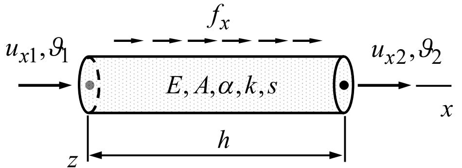
Heat flux through the end-planes is treated by point elements in the same manner as traction on the end-plates by point forces and moments.
