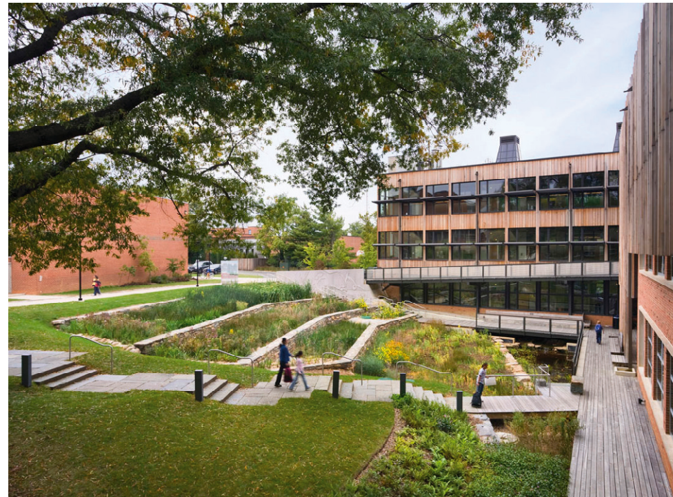
Fig. 4.17 Sidwell Friends Middle School, Washington D.C., USA. Wetlands purifying greywater. The design of these has been integrated into the rest of the landscape.
