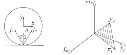
• What's now the wrench cone corresponding to the friction cone  $FC = \left\{k_1 \binom{\mu}{1} + k_2 \binom{\mu}{1} | k_1, k_2 \ge 0\right\}$
