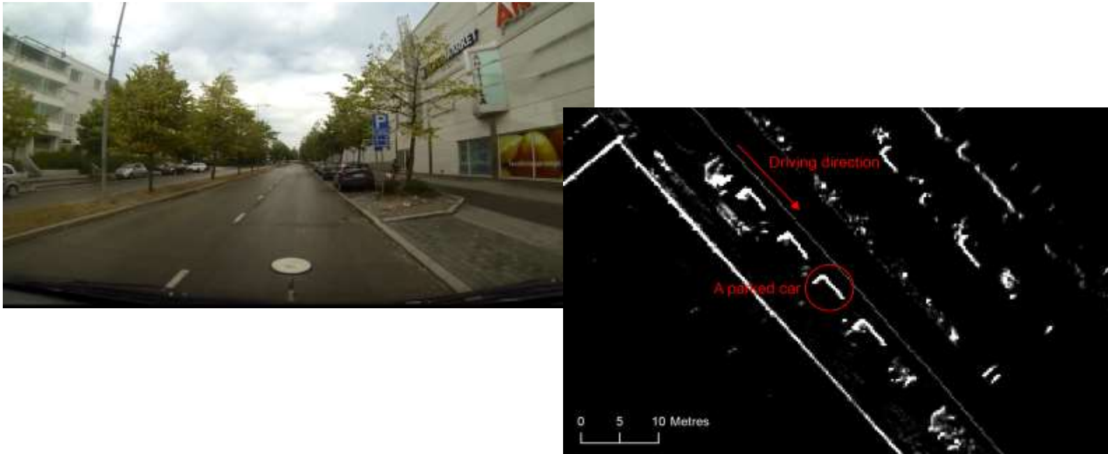
Figure. a) Part of the street Espoonlahdenkatu as recorded on the reference video during data acquisition Drive 1. b) Raster representation of the car-based laser scanner data. The pixel value of each 0.3 \text{ m} \times 0.3 \text{ m} cell corresponds to the number of laser points inside the cell. Parked cars appear as L shaped clusters of bright pixels.
