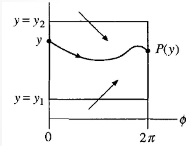
Trajectory starts at a height  $y$  on the left side and intersects the right side at height  $P(y)$ .
