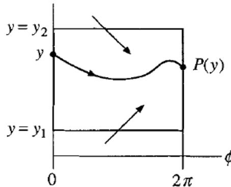
For a trajectory that starts at  $y = y_1, \phi = 0: P(y_1) > y_1$ .
