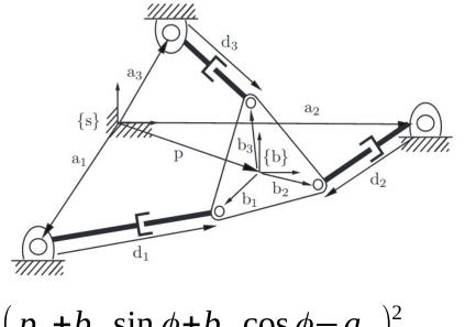
$$d_{i}^{2} = (p_{x} + b_{ix} \cos \phi - b_{iy} \sin \phi - a_{ix})^{2} + (p_{y} + b_{ix} \sin \phi + b_{iy} \cos \phi - a_{iy})^{2}$$
