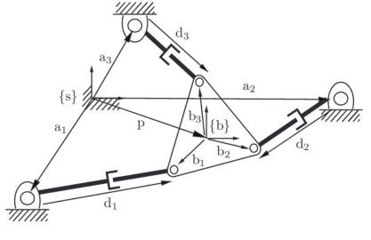
$$d_{i}^{2} = (p_{x} + b_{ix} \cos \phi - b_{iy} \sin \phi - a_{ix})^{2} + (p_{y} + b_{ix} \sin \phi + b_{iy} \cos \phi - a_{iy})^{2}$$
