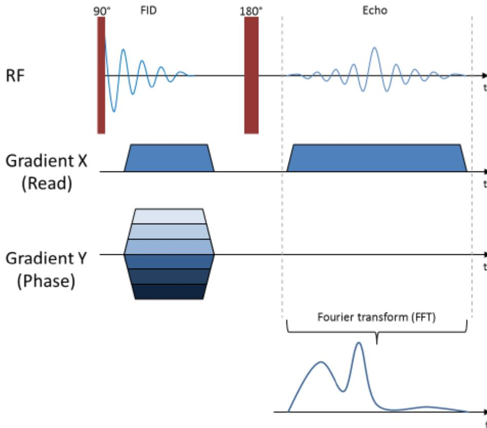
Figure 17: Pulse sequence for experiment Spin Echo 2D
