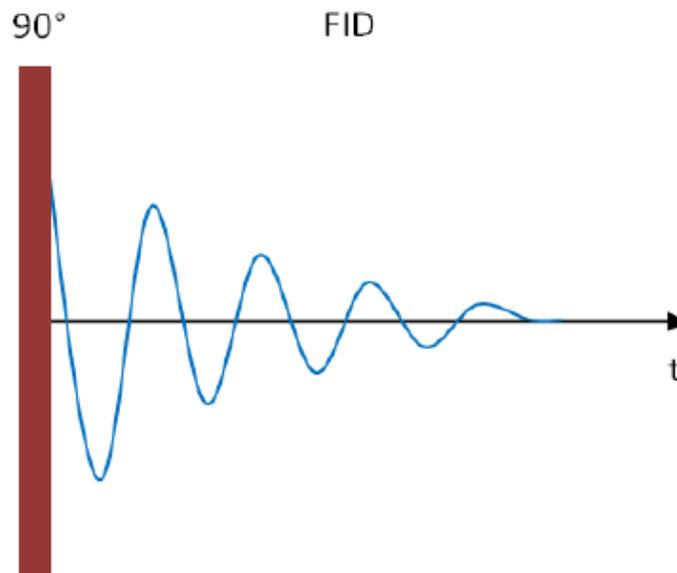
Figure 8: Sequence for the experiment MR excitation angle
