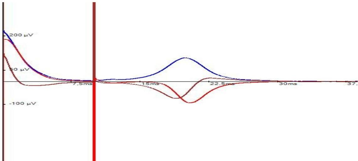
Figure 26: Optimal Spin Echo Signal for 10 mm Oil Sample
