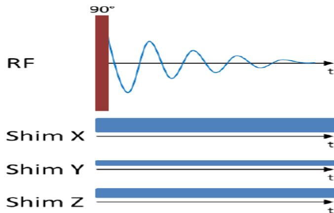
Figure 10: Sequence for experiment B0 homogeneity (magnet shim)
