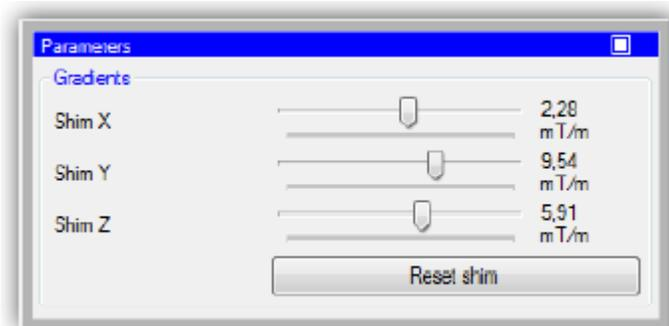
Figure 11: Parameters for experiment B0 homogeneity (magnet shim)
