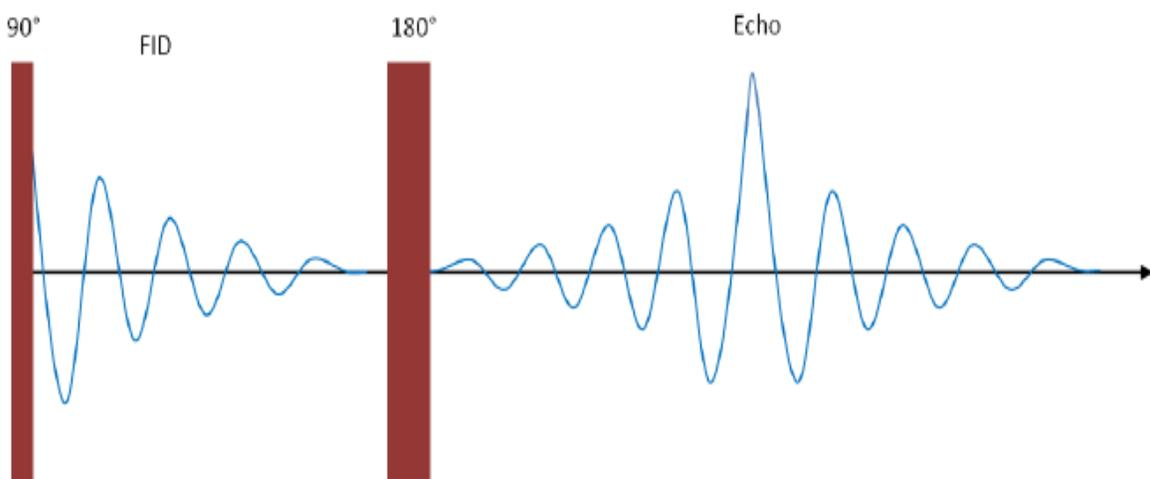
Figure 15: Pulse sequence for experiment Spin Echo
