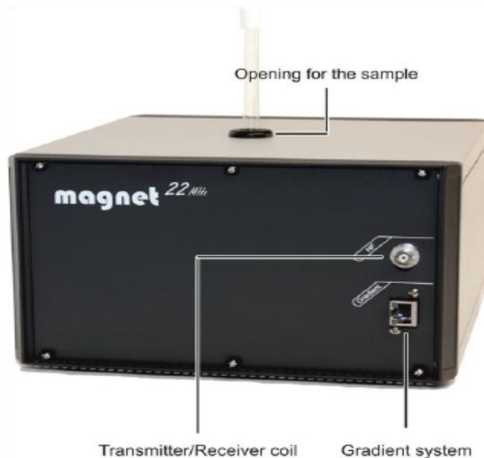
Figure 5: Interfaces of the magnet
