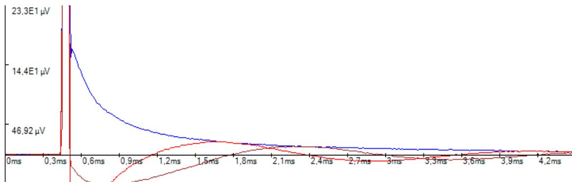
**Figure 21: System frequency matches Larmor frequency**
