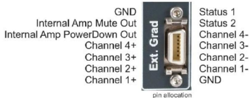
**Figure 4: External gradient amplifier – pin allocation**
