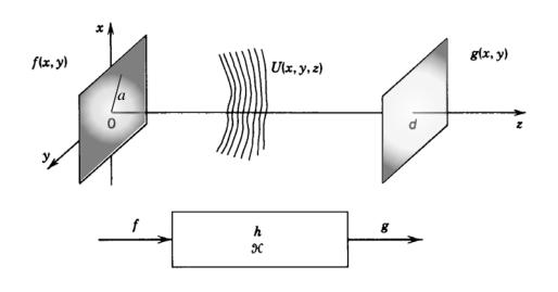
Any linear system can be characterized either by an impulse-response function
