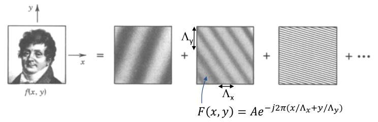
**2D picture:** An arbitrary function f(x, y) may be analyzed as a sum of harmonic functions of different spatial frequencies and complex amplitudes.
