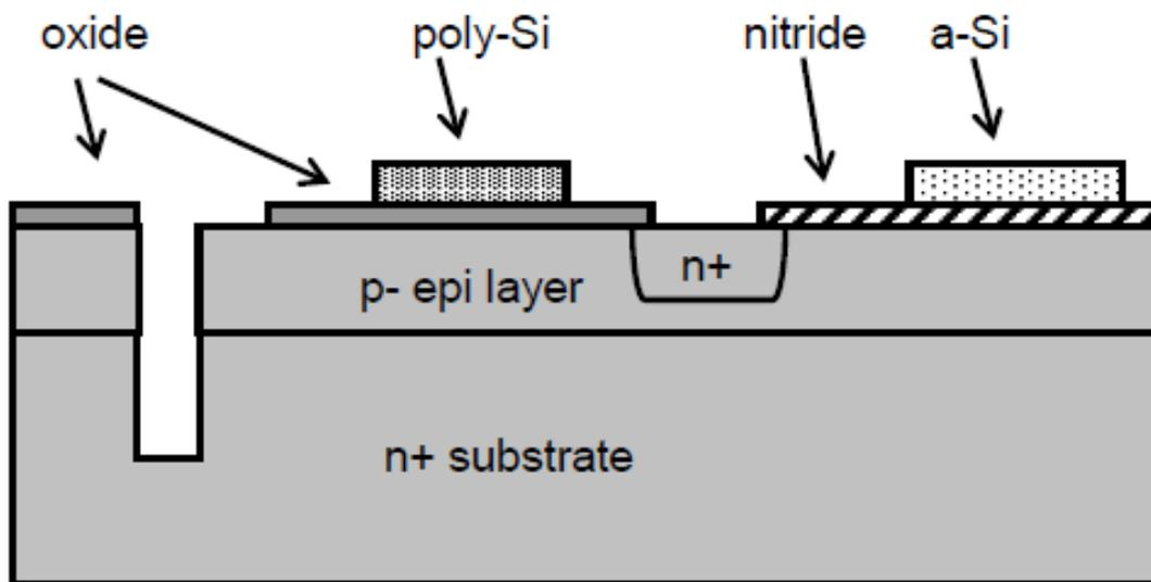
**Q3.** a) Design a step-by-step fabrication process for the device shown below. The n+ doping is done by thermal diffusion.
