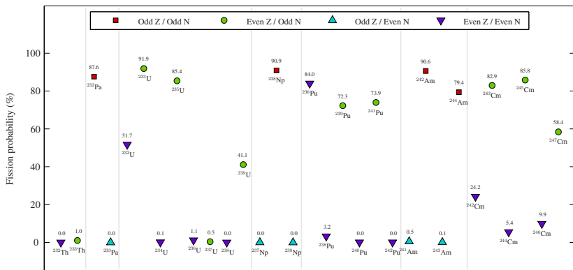
Figure 1: Probability of fission induced by thermal neutrons (Maxwellian energy distribution corresponding to room temperature). If the binding energy released in neutron absorption exceeds the fission barrier, the nuclide can be fissioned by low-energy neutrons. This is more likely to happen with odd-N nuclides, for which the energy release is higher because of the parity effect.
