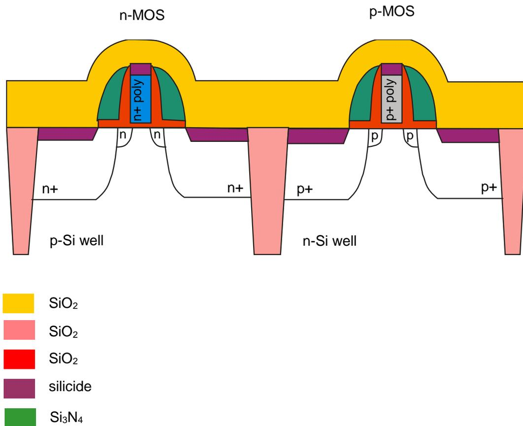
2. Design fabrication process for a thin film MOS transistor given below. Choose materials and thicknesses for all layers. Propose deposition and doping methods. Maximum allowable process temperature is 300 °C. Give top view of the transistor. How small is it (length and width)? (2p)
