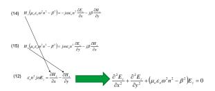
**Electromagnetic Model of Light Propagation**
