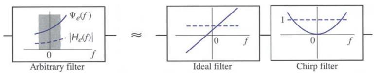
Gaussian chirp filtering of an unchirped Gaussian pulse:
