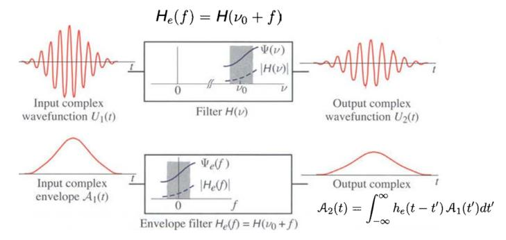
An ideal *non-disturbing filter* introduces constant attenuation and time delay  $\tau_d$  of each frequency component:  $H_e(f) = H_0 \exp(-j2\pi f \tau_d)$ .
