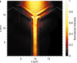
• Plasmonic waveguide mode is much better confined to the guiding material than would be the case in dielectric-based waveguides.
