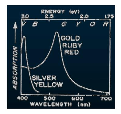
Au nanoparticles for red coloration Ag nanoparticles for yellow coloration
