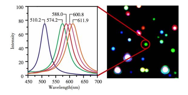
Single Ag nanoparticle resonant Rayleigh scattering spectrum in various solvent environments (left to right): nitrogen, methanol, 1-propanol, chloroform, and benzene.
