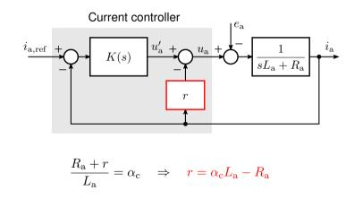
This controller structure could also be represented as a state feedback controller with integral action and reference feedforward.
