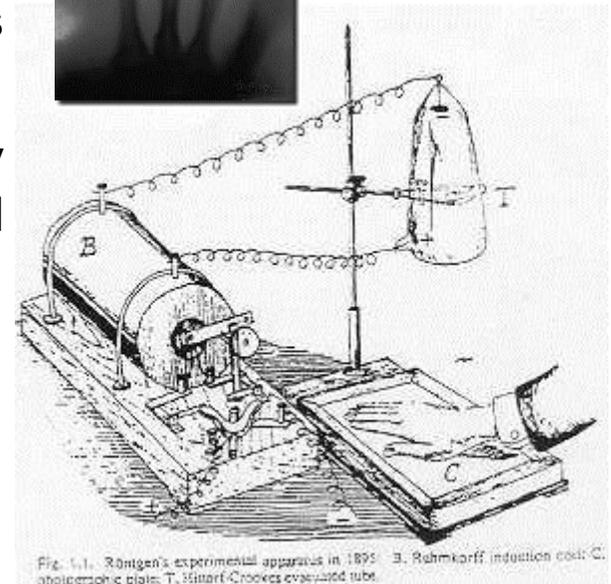
Fig. 1.1. Röntgen's experimental apparatus in 1895. B. Ruhmkorff induction coil; C. photographic plate; T. Hittorf-Crookes evacuated tube.
