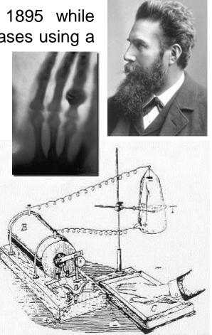
Fig. 1.1. Romgen's experimental apparatus in 1895 B. Rohmkorff induction cost: C. oholographic plaim, T. Hinterf Crookes evacuated tube.
