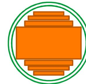
Cross section of the iron core and the windings
