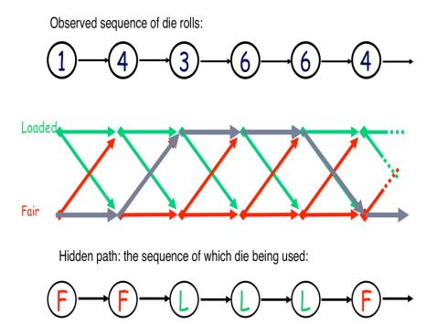
$$V_{\text{loaded}}(5) = E_{\text{loaded}}(6) \cdot \max \begin{cases} V_{\text{loaded}}(4) \cdot T_{\text{loaded,loaded}} \\ V_{\text{fair}}(4) \cdot T_{\text{fair,loaded}} \end{cases}$$
