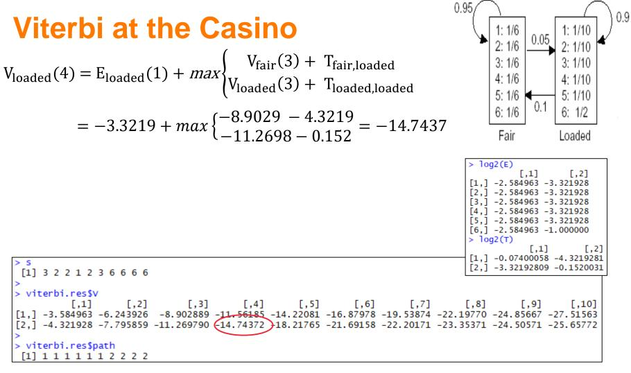
$$V_l(i+1) = E_l(s_{i+1}) + \max_k(V_k(i) + T_{kl})$$
