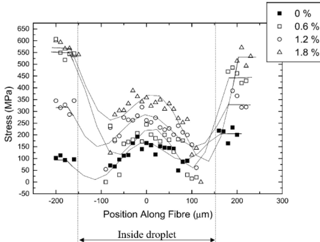
Axial stress along fibre, measured using Raman spectroscopy
