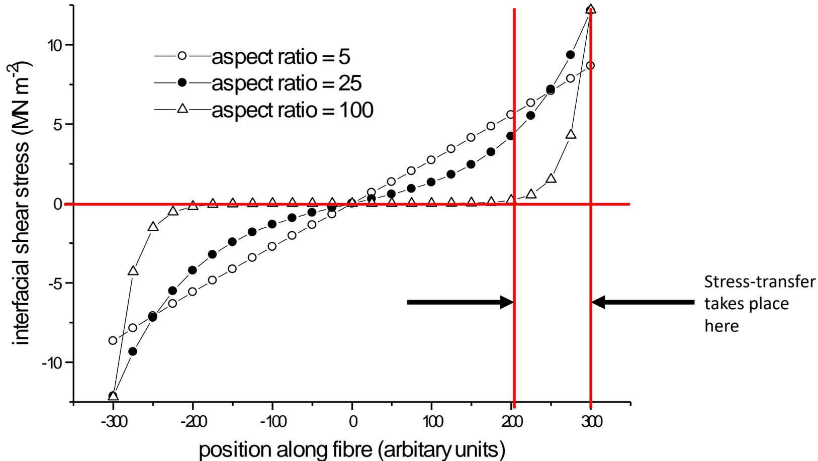
Assumptions: fibre modulus: 50 GPa; matrix modulus: 3.5 GPa; axial strain: 0.5%
