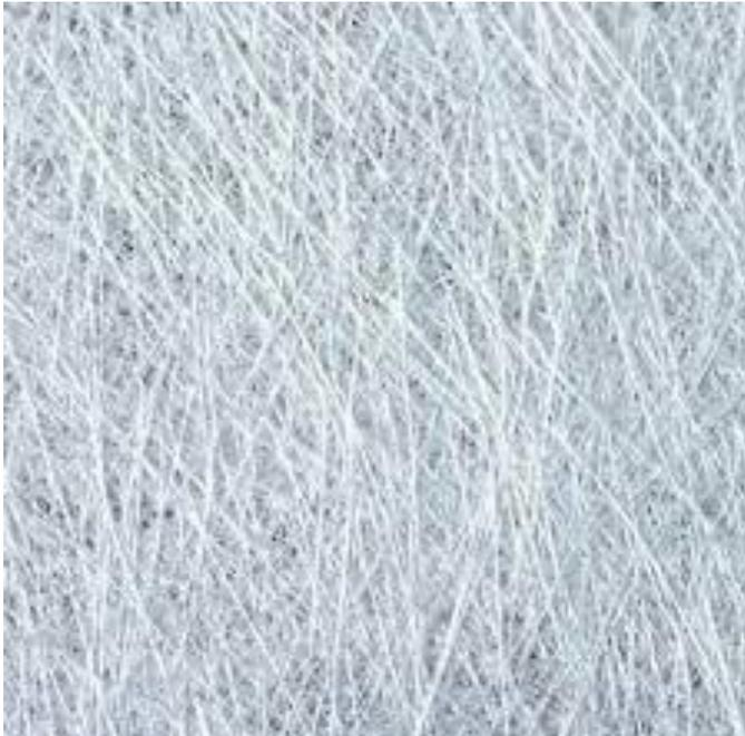
Above: Chopped Strand Mat (CSM) reinforcement. A 2-D random arrangement of fibres
