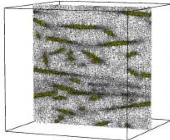
Computer model consisting of 150 fibres with an aspect ratio of 37. Volume fraction 8% (Source: ETH Zurich:
