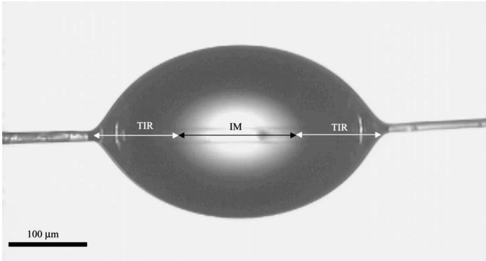
Microdroplet test: hemp fibre embedded in epoxy
