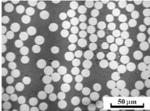
Figure 2. (a) Overall aspect of the microstructure of the composites, showing a regular fiber spacing and low void content; (b) Detail of the fiber distribution inside a tow.
