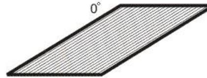
One individual ply with fibre reinforcement
