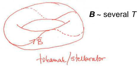
In fusion energy research, the VERY hot plasma is kept away from the vessel walls by magnetic field.
