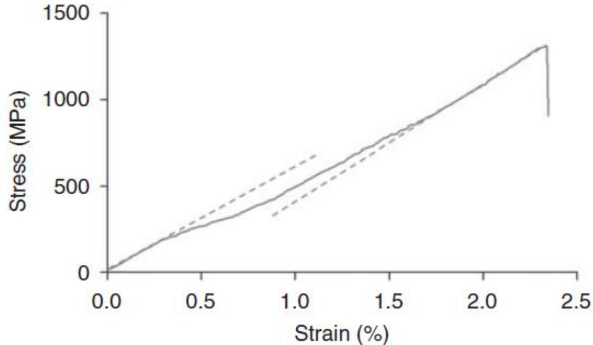
*Figure 1. Typical stress–strain curve of an elementary flax fiber.*
