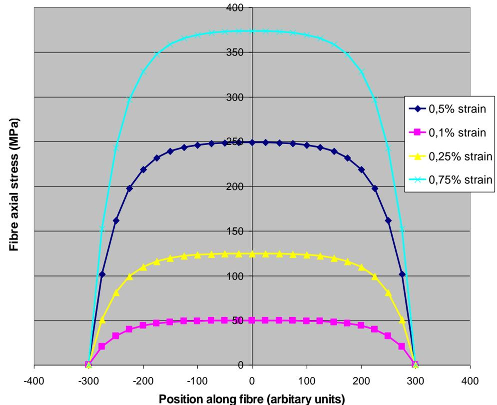
Theoretical build up of fibre axial stress following a Cox type shear lag mechanism ( $E_f = 50$  GPa;  $E_m = 3.5$  GPa;  $s = 50$ )
