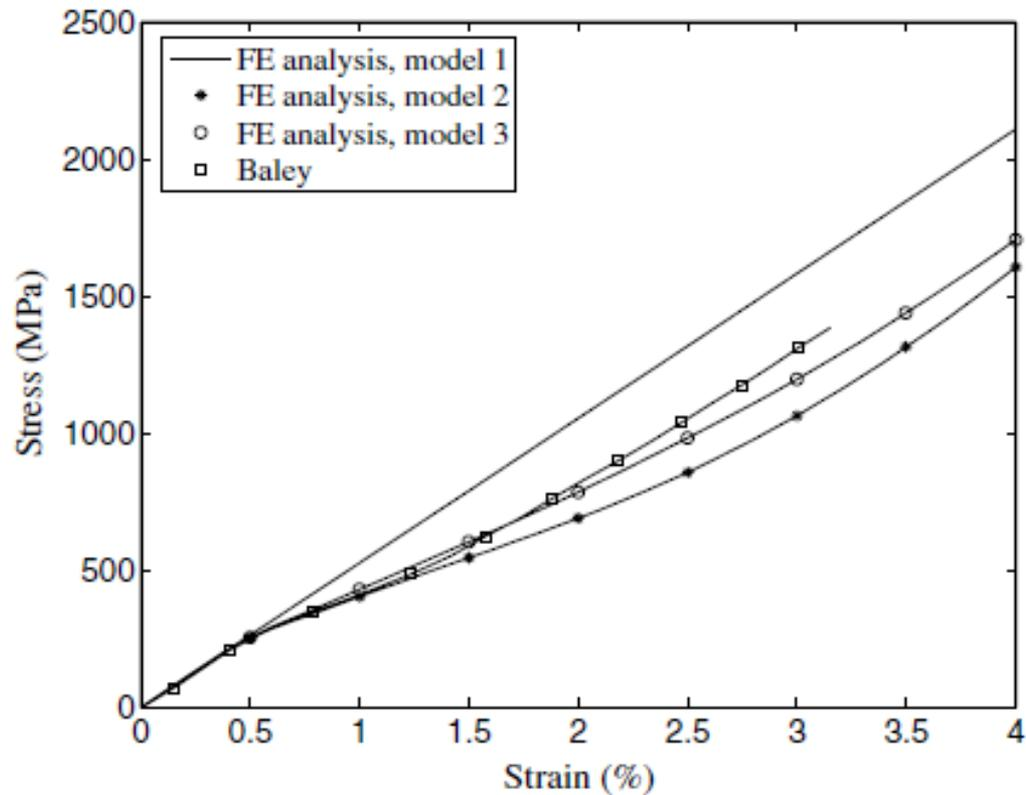
Fig. 7. Tensile behaviour of the elementary fibre.
