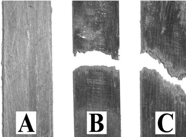
Increased adhesion reduces interfacial de-bonding and results in a change in the fracture behaviour: ductile to brittle
