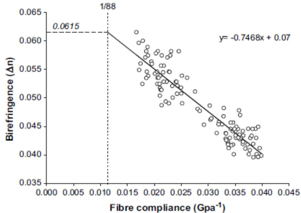
Greater orientation leads to stiffer fibre – good for composite reinforcement
