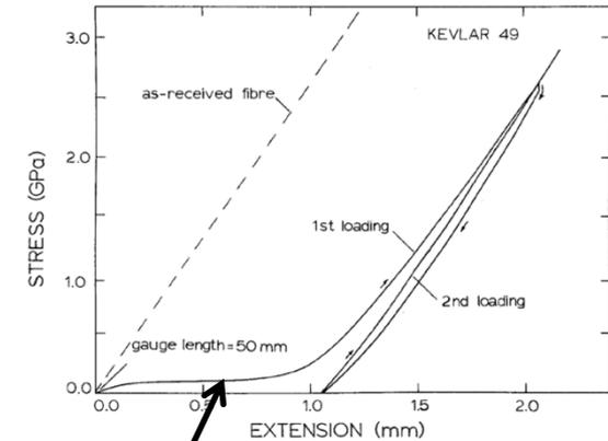
Figure 7 Tensile stress–elongation curve of Kevlar 49 fibre previously compressed ~ 3% due to matrix shrinkage.
