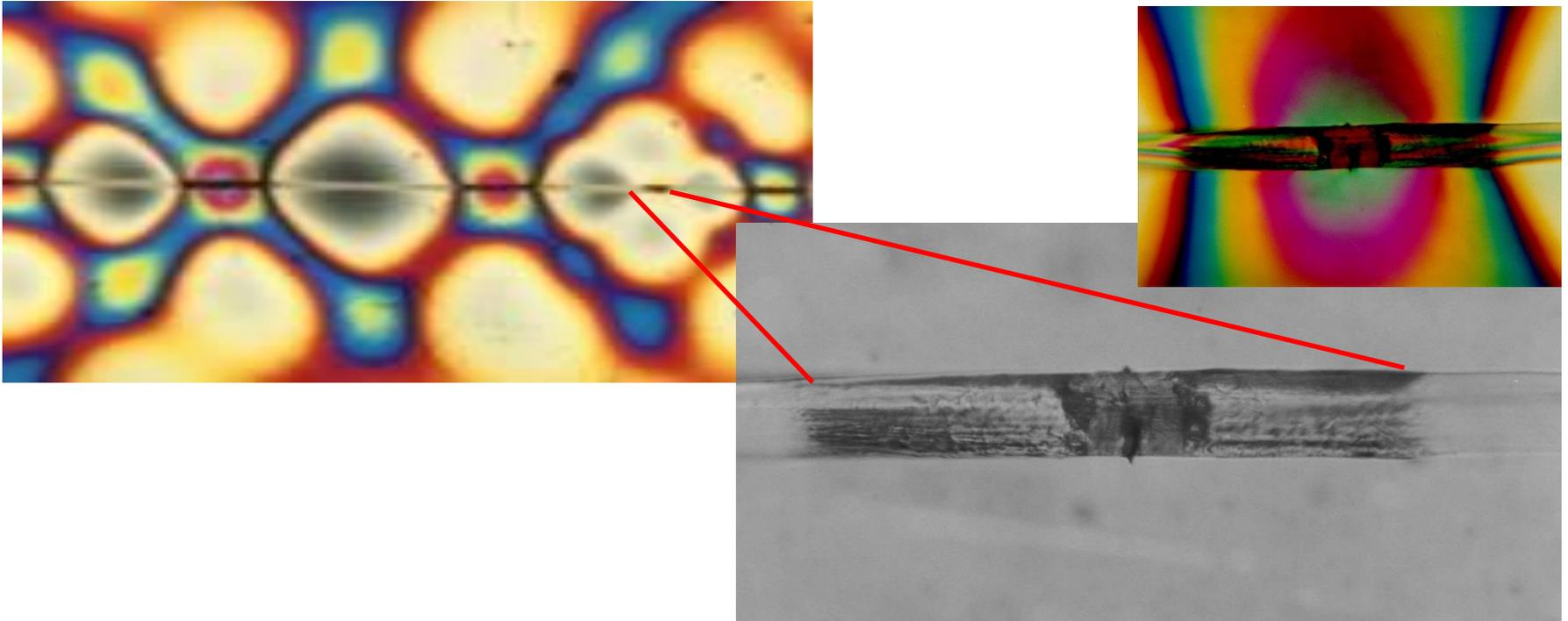
Polarised light micrograph of a failed single filament composites showing fibre-matrix de-bonding in regions of high shear-stress concentration adjacent to fibre defects (and fracture)
