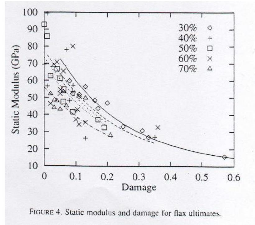
FIGURE 4. Static modulus and damage for flax ultimates.
