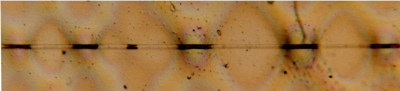
Fragmented flax fibre in an epoxy matrix SFC
