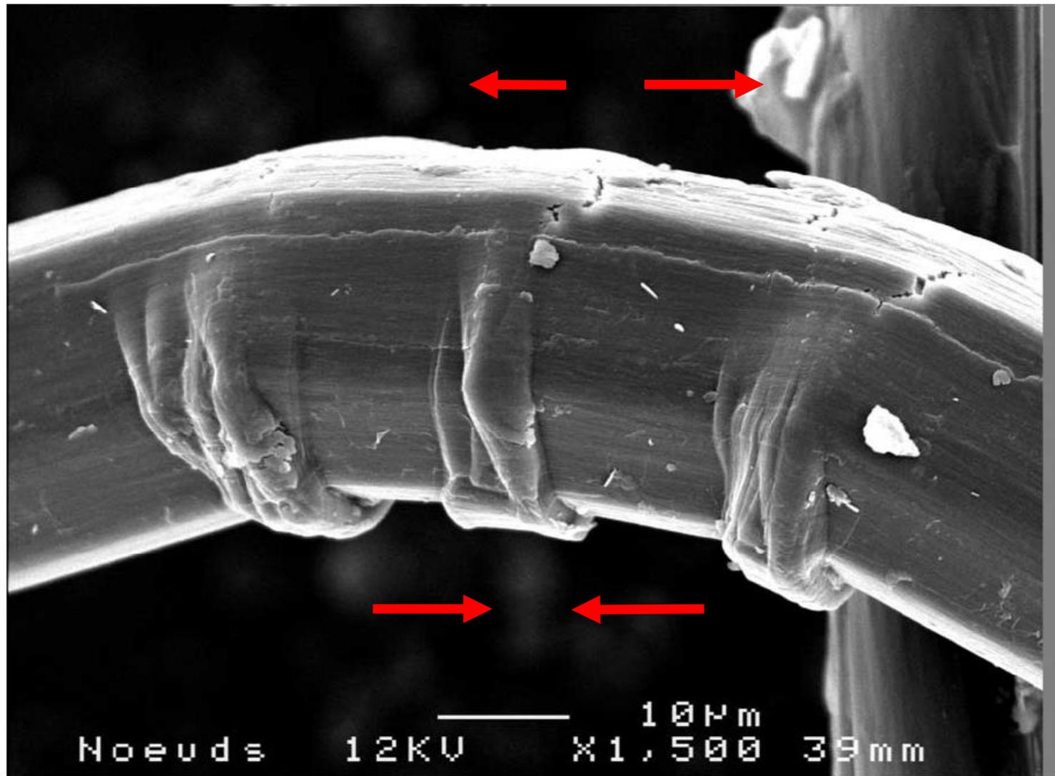
Figure 2 Bending of a flax fiber with buckling of cell walls.
