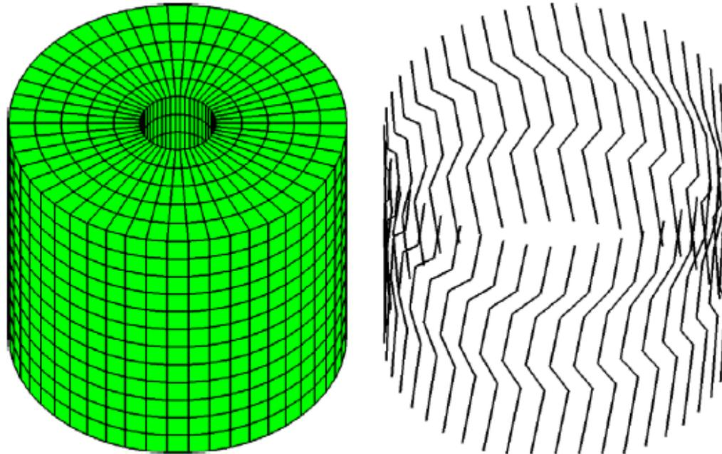
Fig. 4. Part of an FE model with dislocations, hemicellulose to the left and the embedded cellulose with dislocations to the right. Note that only the outermost truss elements are shown.
