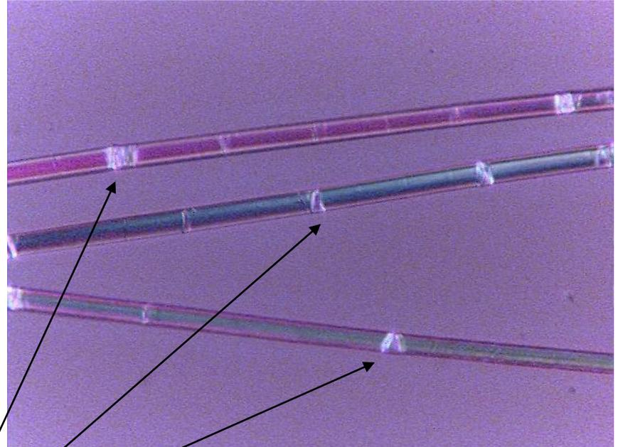
Fibre defects in flax fibre; points of weakness, seen under polarised light
