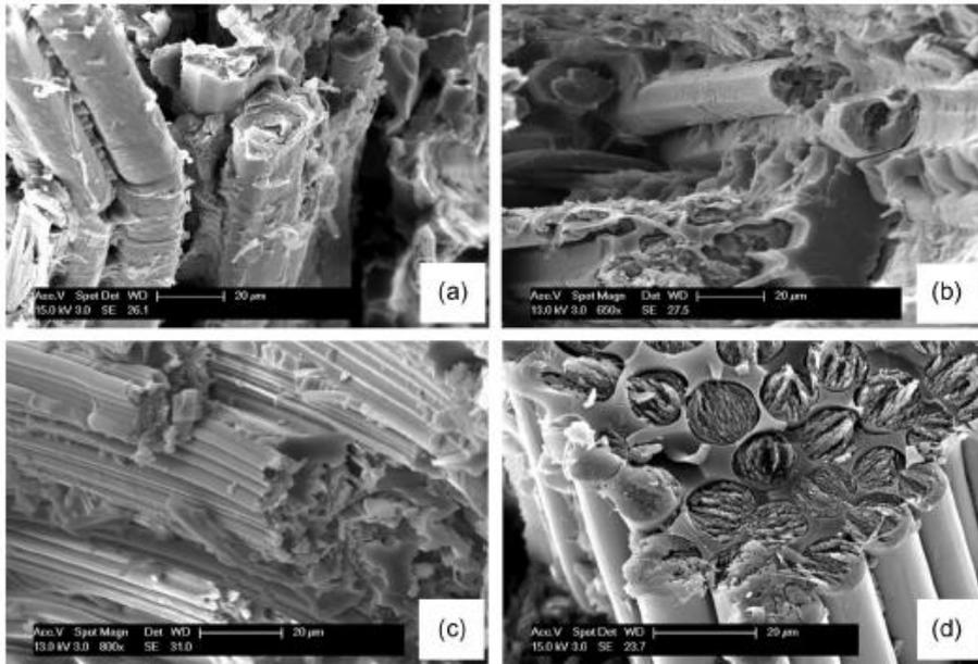
Fig. 4. Longitudinal tension fracture surfaces of (a) Flax1, (b) Flax2, (c) Flax3 and (d) Cellulose reinforced specimens.
