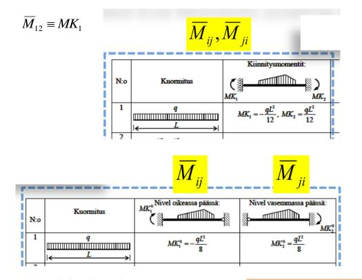
The stiffness equation relating the end-moments to the end-displacements
