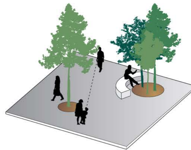
Solitary trees planted between paving with grates covering the soil. High stem trees are used to preserve visibility.
