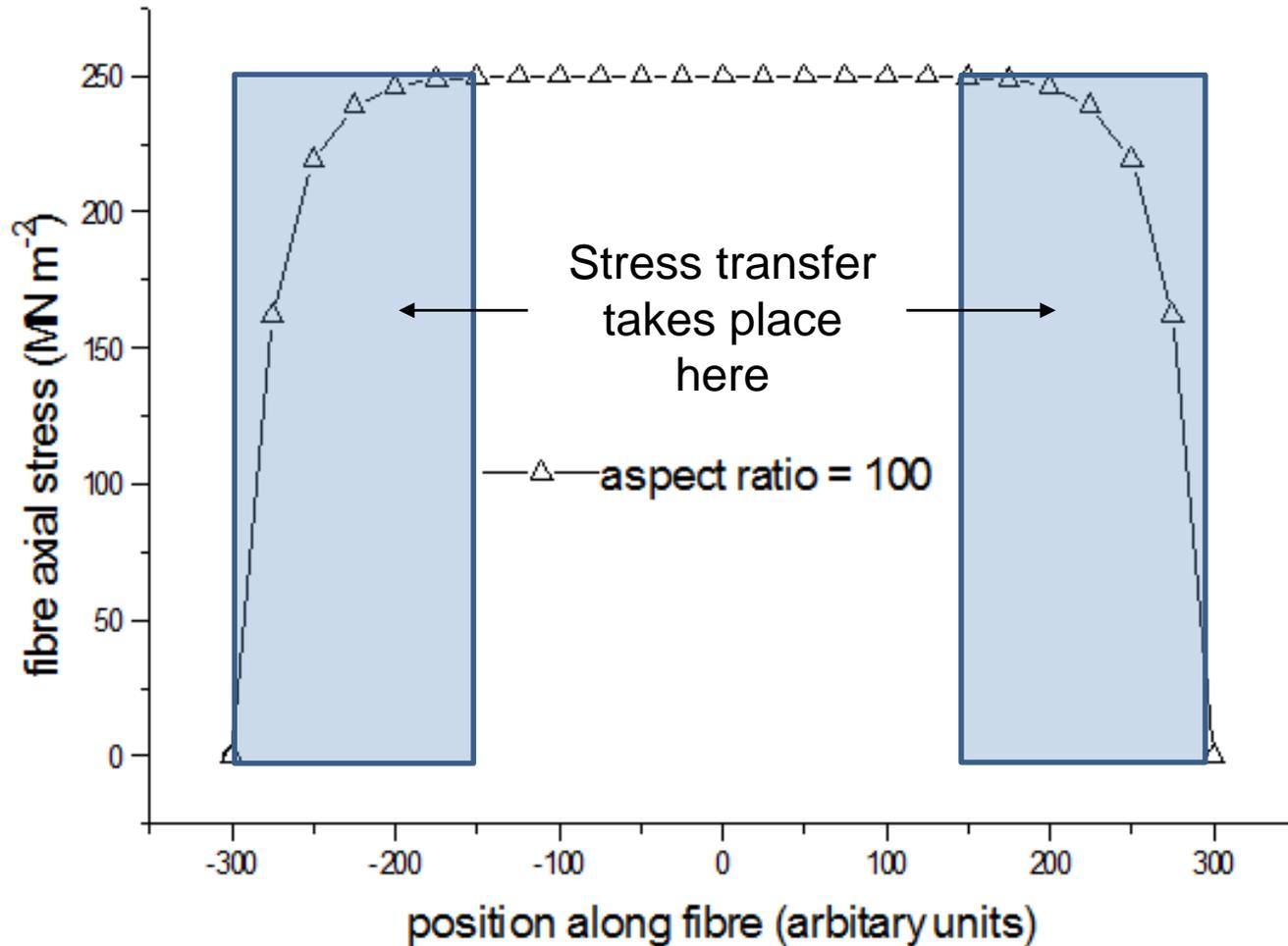
(Assumptions: fibre modulus: 50 GPa; matrix modulus: 3.5 GPa; axial strain: 0.5%)
