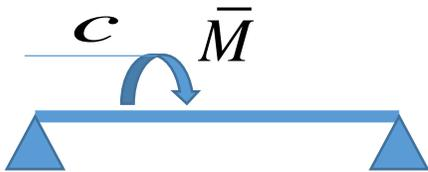
$$\alpha_{ij}^o = -\frac{\bar{M}k \cos k(L-c)}{P \sin kL} + \frac{\bar{M}}{PL}, \quad \alpha_{ji}^o = -\frac{\bar{M}k \cos kc}{P \sin kL} + \frac{\bar{M}}{PL}$$
