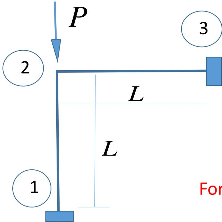
$$\begin{cases} M_{21} = A_{21}\varphi_{21} + B_{12}\varphi_{12} - C_{12}\psi_{21} + (MK)_{21} \\ M_{23} = a_{23}\varphi_{23} + b_{32}\varphi_{32} - c_{23}\psi_{23} + (MK)_{23} \end{cases}$$
