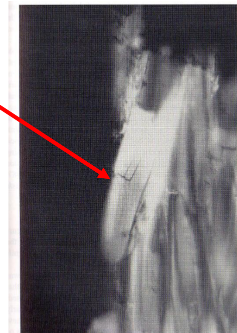
Figure 7.18 Crack-stopping in a fractured rotor blade. The orientation of the secondary cracks corresponds to the microfibrillar orientation of the middle layer of the secondary cell wall ( \times 990 , polarised light.) (© BRE.)
