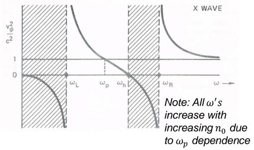
The resonance and cut-off frequencies divide the dispersion diagram into propagation and nonpropagation zones.
