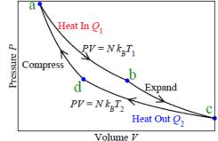
Fig. 5.3 Carnot cycle P-V diagram. The four steps in the Carnot cycle:  $a \rightarrow b$ , heat in  $Q_1$  at constant temperature  $T_1$ ;  $b \rightarrow c$ , expansion without heat flow;  $c \rightarrow d$ , heat out  $Q_2$  at constant temperature  $T_2$ ; and  $d \rightarrow a$ , compression without heat flow to the original volume and temperature.
