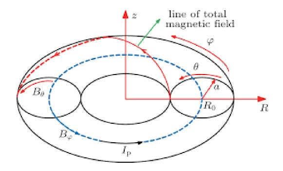
Toroidal angle:  $\varphi$ Poloidal angle:  $\theta$ Toroidal field:  $B_{\varphi}$ Poloidal field:  $B_{\theta}$ Major radius: RMinor radius: r(a)Magnetic axis at  $R = R_0$
