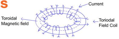
When the axial field is turned into a toroidal one, it becomes non-uniform.
