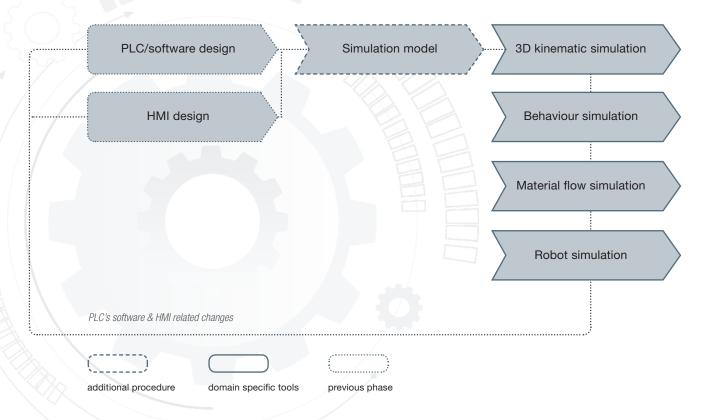
Based on practical experience, the 3D simulation model created and used by virtual engineering is taken as a base in order to use it for VC. In the market, several tools provide required functionalities to prepare the 3D simulation model and to conduct VC, e.g. DELMIA, Process Simulate, NX-MCD, RF::SGEdit, RF::YAMS etc.
