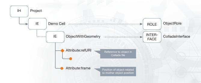
COLLADA is an XML-based data format with a modular structure enabling the definition of libraries of visual and kinematic elements. The most important feature of AutomationML is the clear identifiability of objects in COLLADA files, which allows the integration of these files into AutomationML. Several data objects within a COLLADA file have a unique identification (ID) like geometries, visual scenes, kinematic models and kinematic scenes.
