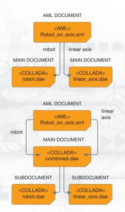
Naturally, an InstanceHierarchy may contain more than one Internal-Element with a geometry assigned to it. There are different ways to define the relationship between different objects. The two possibilities are shown in the figure on the left. The relationship between the linear axis and the robot can be defined in a common COLLADA file and then referenced. The other option is to reference two separate COLLADA files and define the relationship in the AutomationML file.
