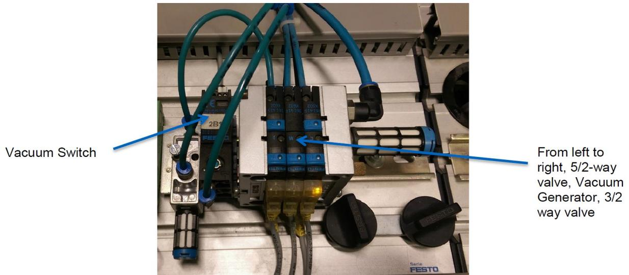
Figure 9 Pneumatic valves subsystem
