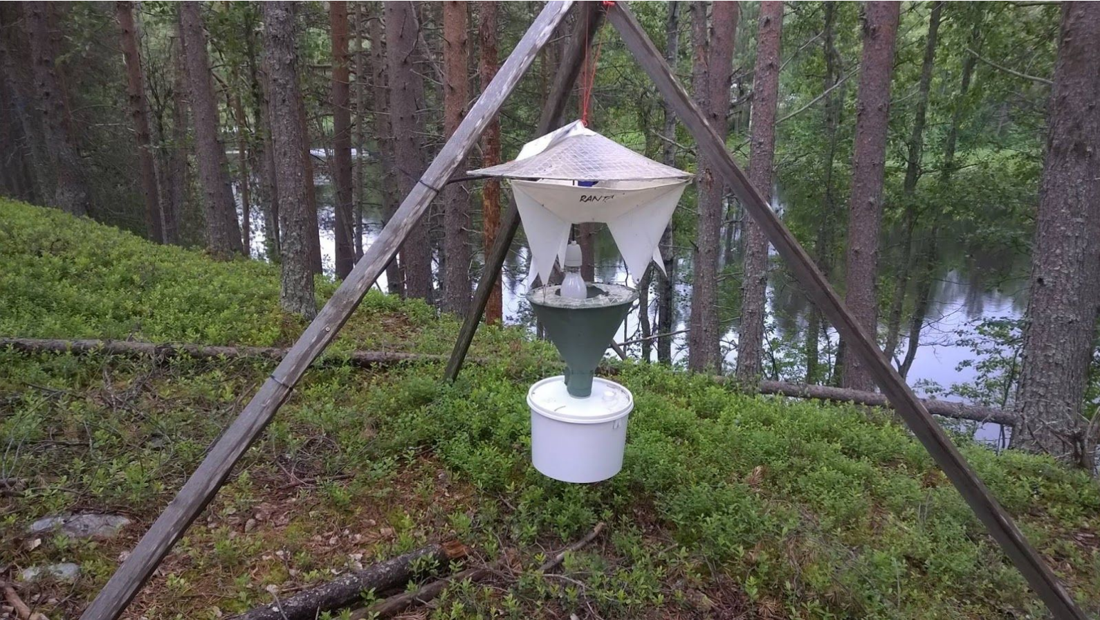
Figure 2. A self-built, analog moth trap (Leinonen et al., 2016).
