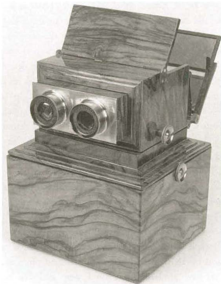
Figure 4.1 Achromatic stereoscope. 90 × 120 cm, ca. 1860. Smith, Beck, and Beck, London. By kind permission of Gerhard Kemner.
