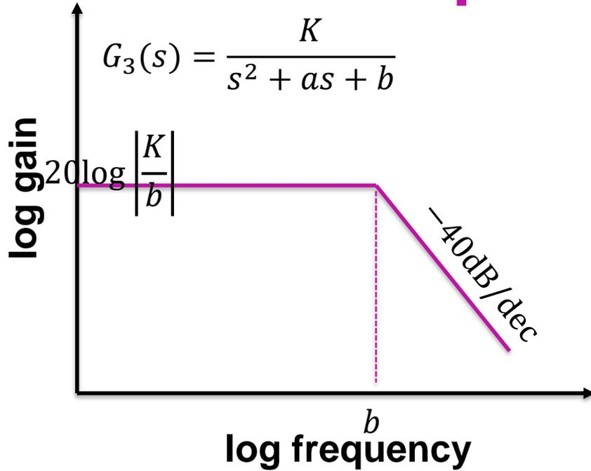
Phase: from zero to  $-180$  deg. in range of  $0.1b$  to  $10b$
