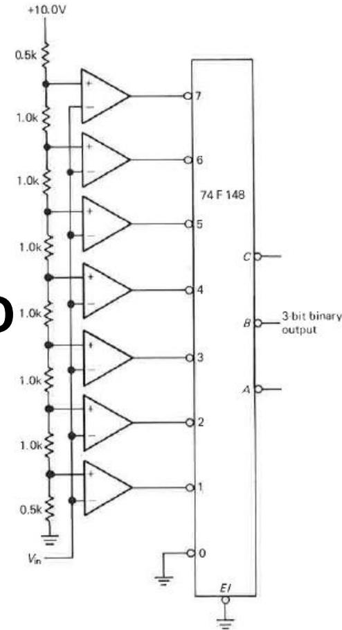
Pic. by Horowitz & Hill in “The art of electronics” on p. 621 Figure 9.49. Parallel-encoded (“flash”) A/D converter (ADC).
