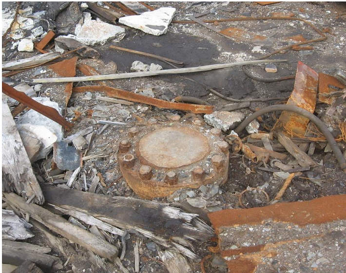
The borehole, welded shut
