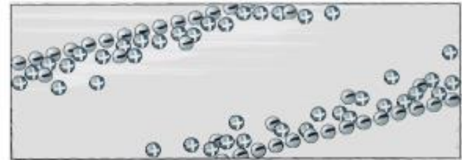
b) diffuse layer of counterions near surface
