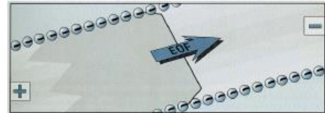
c) E applied, bulk flow towards cathode
