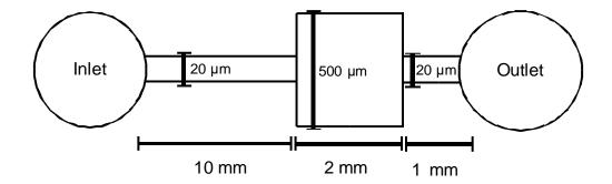
c) The chip inlet is connected to a pressure pump with tubing that has circular cross section and inner radius of 1 mm. The length of the tubing however varies from experiment to experiment between 10 cm and 30 cm. Does this variation have a big effect on the flow rate?
