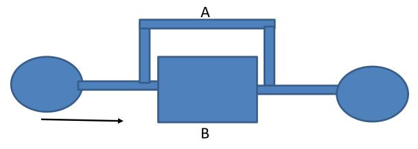
Also, note that in a series, all components have the same flow through them, but this is NOT the case with a parallel configuration.
