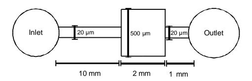
c) The chip inlet is connected to the pressure pump with tubing that has circular cross section and inner radius of 1 mm. The length of the tubing however varies from experiment to experiment between 10 cm and 30 cm. Does this variation have a big effect on the flow rate?
