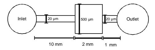
**Step 1:** calculate the hydraulic radius
