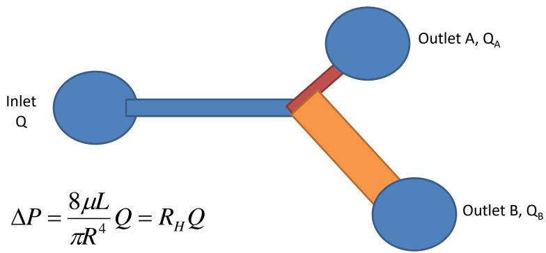
Orange channel: all dimensions are doubled compared to the red channel.
