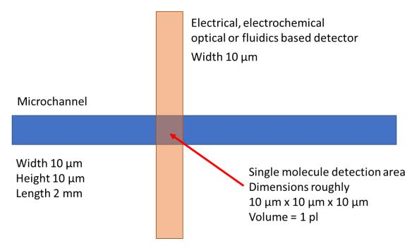
Single molecule detection strategy based on defining a suitably small volume by the "intersection" of the detector (=where the molecules would be detected) with the channel (=where the molecules are). (with the dimensions given in this calculation there would still be some work to do).
