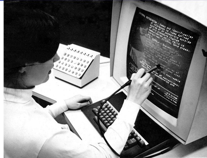
IBM 2250 Model 4, including light pen and programmed function keyboard.
