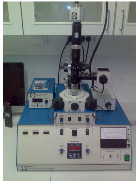
Planar Surface Preparation for SEM Cross Section Viewing
