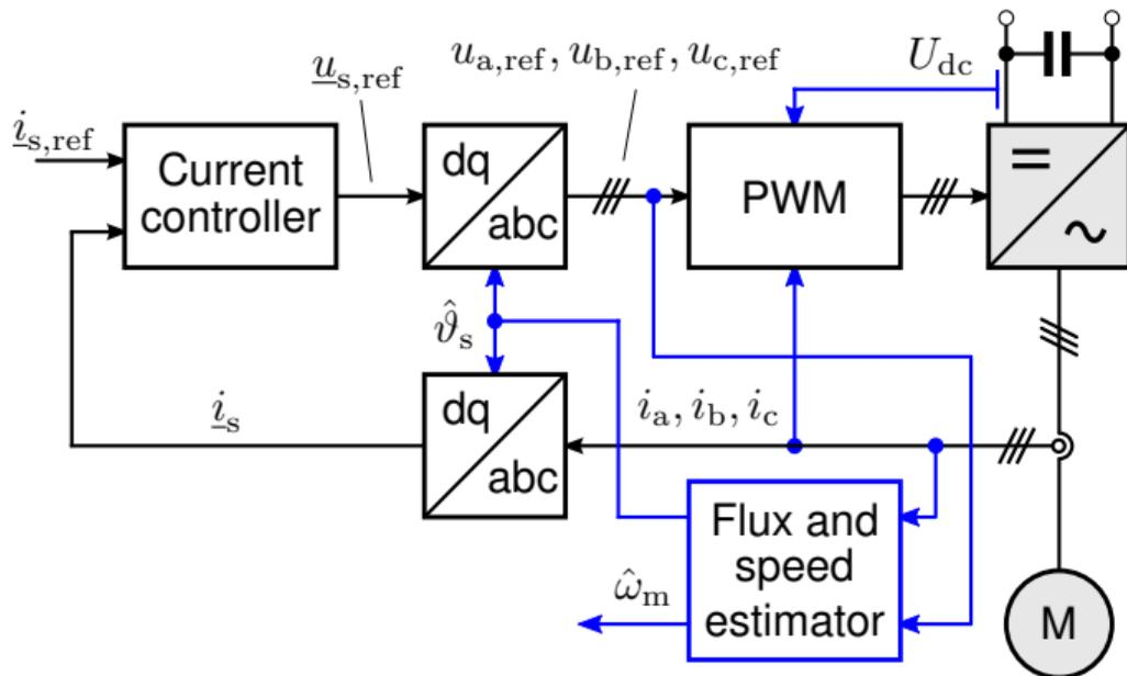
The inverter nonlinearities can be approximately compensated for as  $u'_{a,ref} = u_{a,ref} + \Delta u \text{sign}(i_a)$ , where  $u'_{a,ref}$  is the compensated voltage reference and  $\Delta u$  is the compensation magnitude (typically a few volts). The compensation is used for the b- and c-phases as well.
