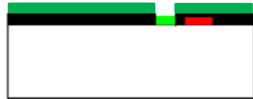
Deposition of palladium electrode by evaporation process
