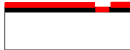
Deposition of gold electrode by evaporation process
