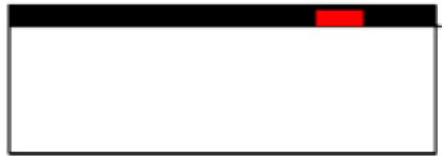
Deposition of photoresist
