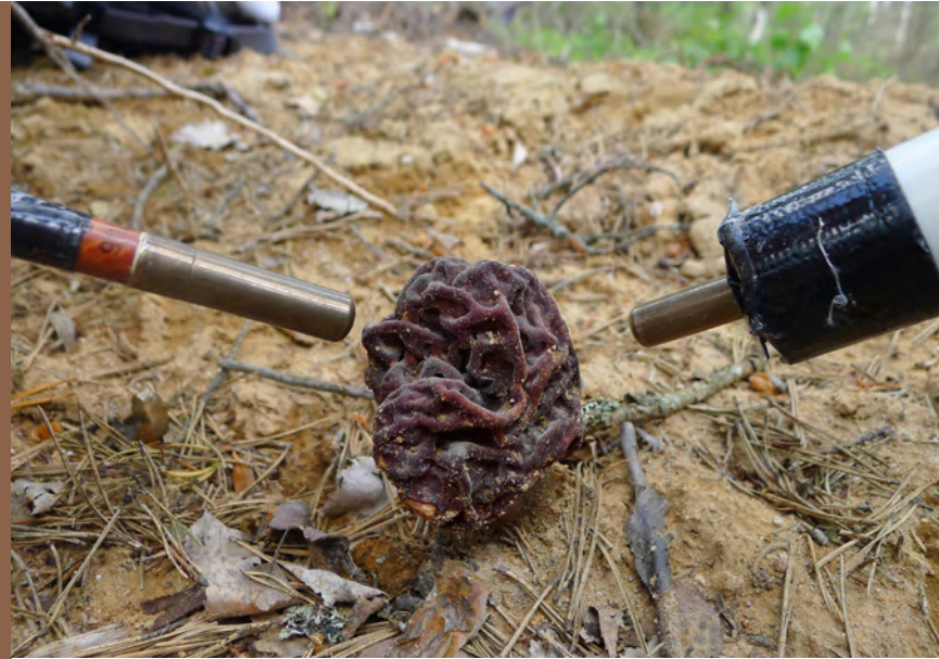
Testing mushrooms for radioactivity at the Palmutto uranium deposit. Photo by Martin Howse.
