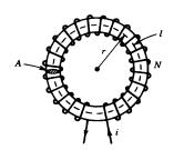
Measurements have been carried out by feeding the primary coil with a current i=1\*sin(2\*pi\*t) A. The measured induced voltage in the secondary coil was u=0.1\*cos(2\*pi\*t-0.2) V. Compute the magnetic field strength H along the average perimeter of the toroidal and the average magnetic flux density B through it. Plot B as a function of H.
